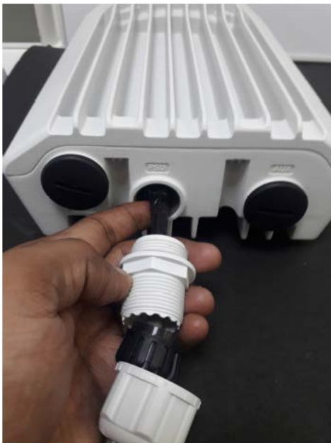
Figure 117: Removing the latch of the RJ45 plug
