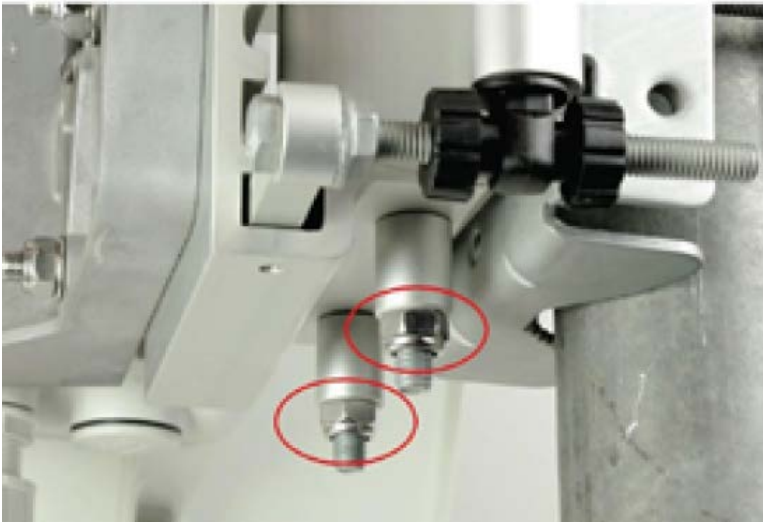
Figure 94: Two Nyloc screws in the azimuth
