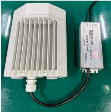
Figure 123: Connecting the output side of AC/DC PSU
