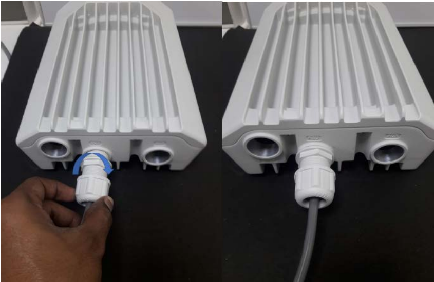
Figure 114: Rotating the gland
