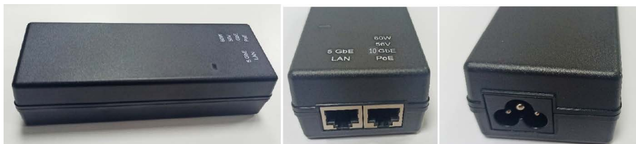
Figure 36: PoE power supply to V3000 or V5000
