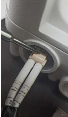
Figure 150: Pulling the bale clasp (latch)
