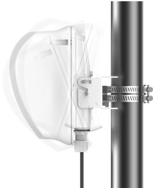
Figure 80: Using the adjustable bracket knob for alignment
