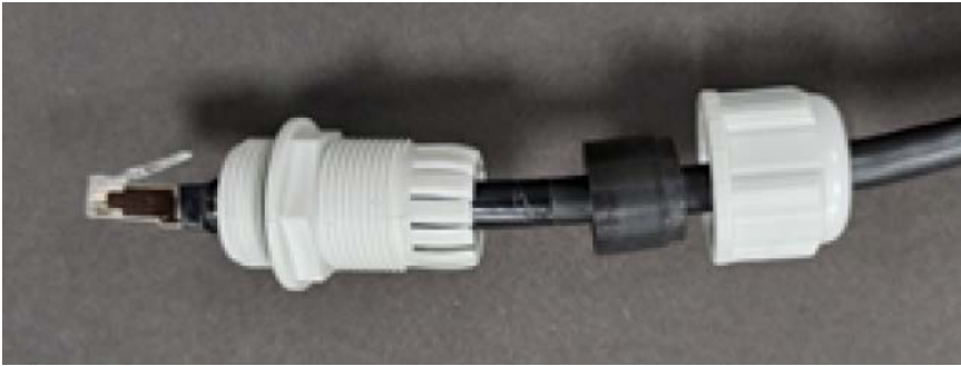
Figure 112: Fixing the gland nut
