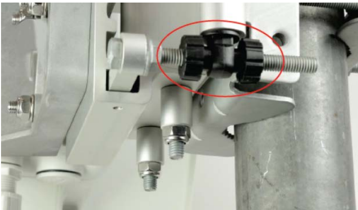
Figure 96: Moving the azimuth adjuster
