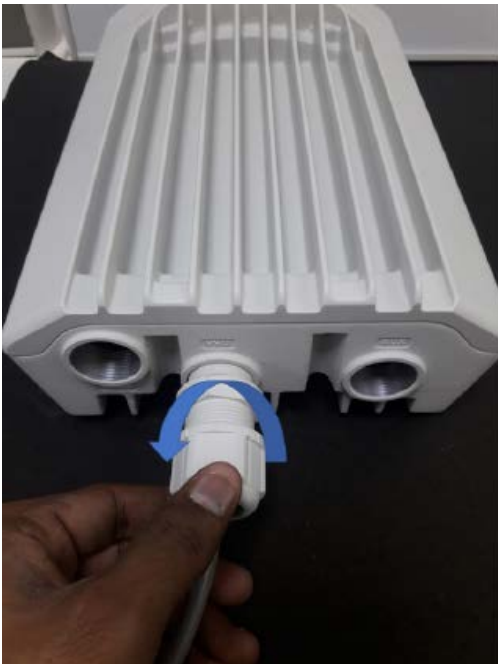
Figure 115: Removing the cable clamp
