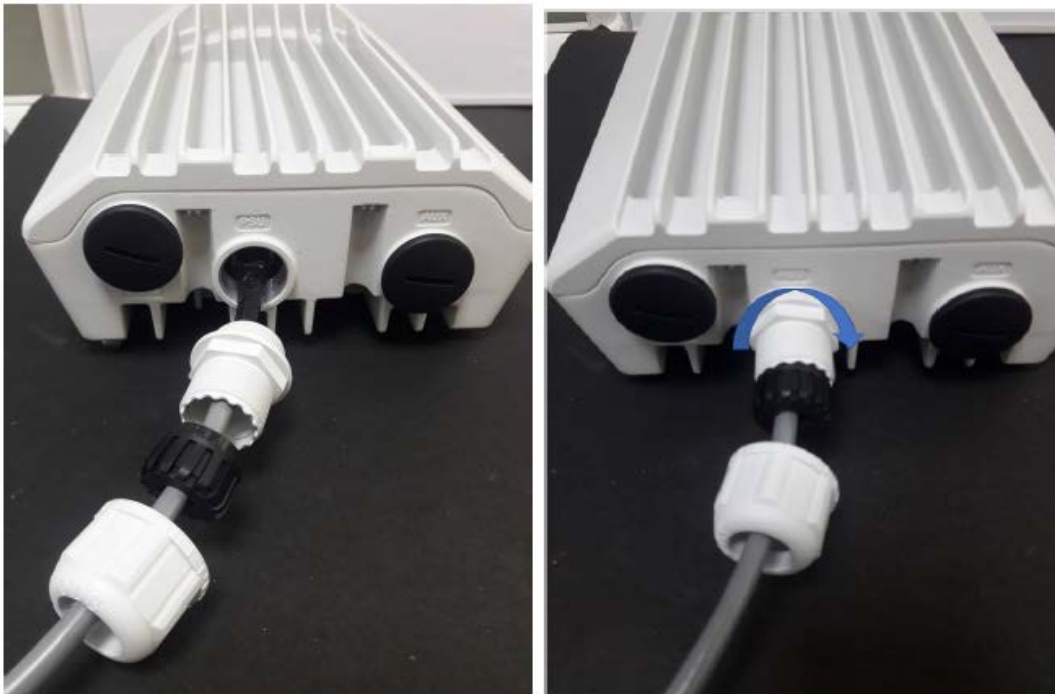
Figure 113: Connecting the RJ45 plug
