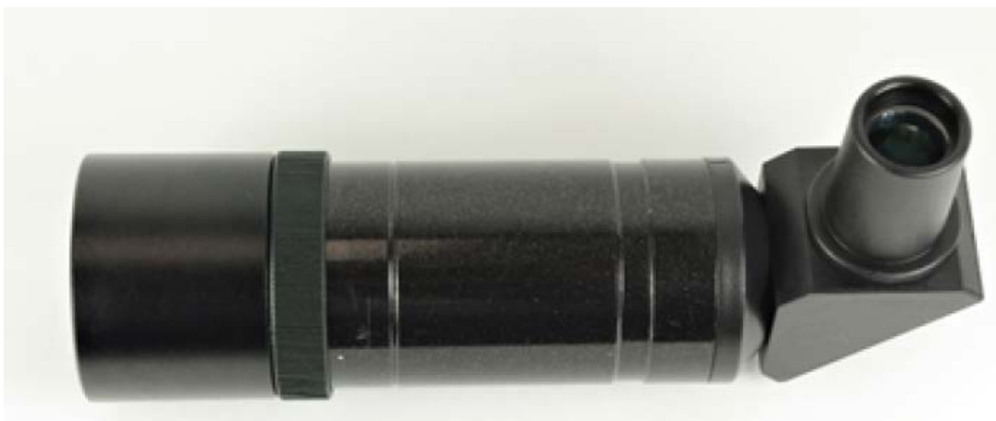
Figure 27: Typical alignment telescope
