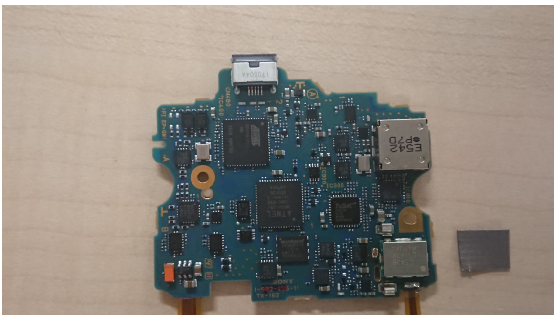
Fig.12: Removed the electromagnetic absorber sheet
