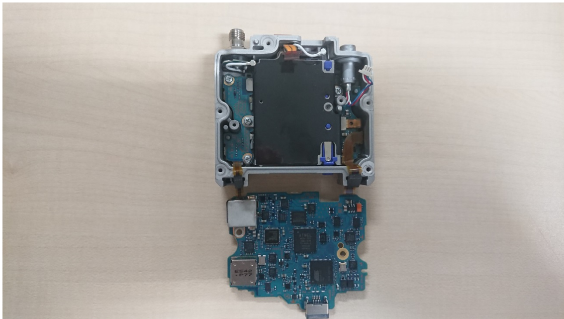
Fig4: Removed the board TX-162, main block
