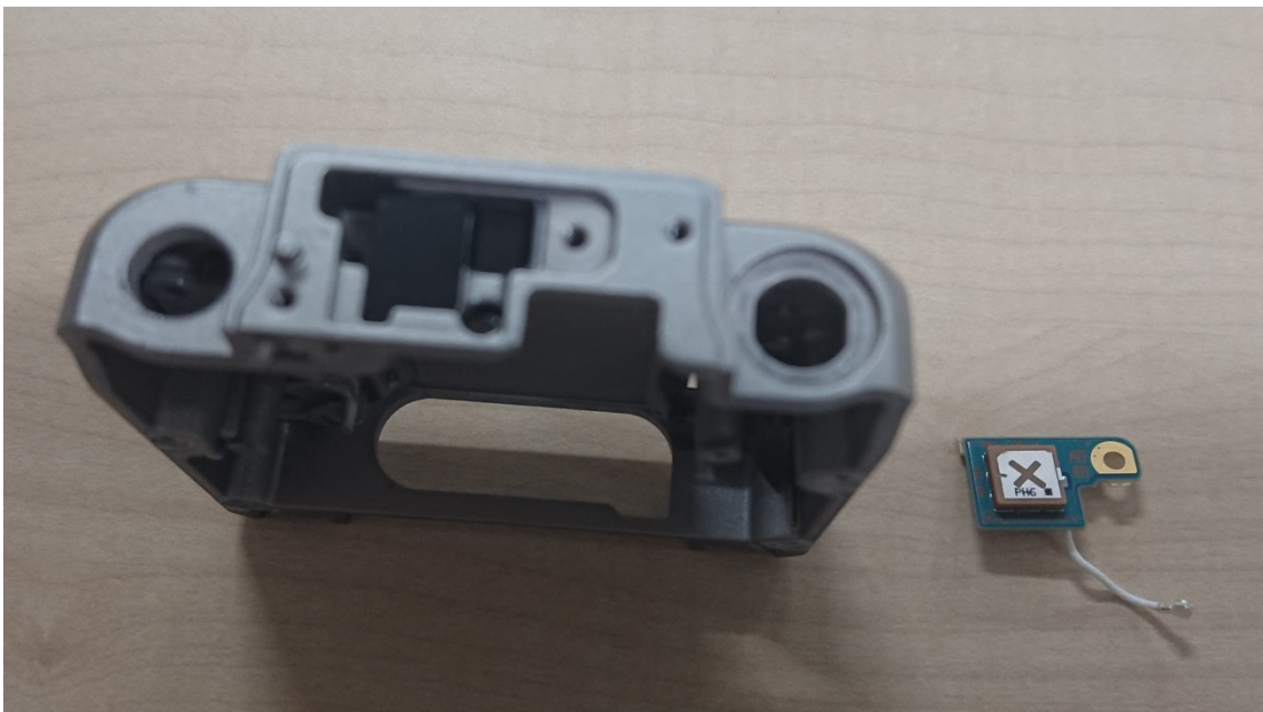
Fig16: Removed the board RM-251
