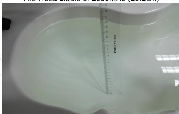
The Head Liquid of 3700MHz (15.6cm)
