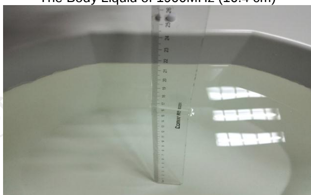
The Body Liquid of 2600MHz (16.5cm)
