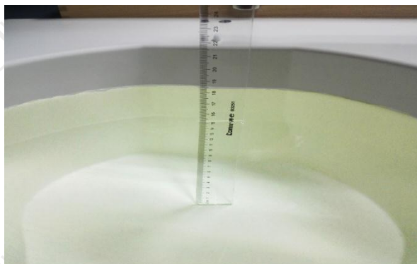
The Body Liquid of 1800MHz (15.2 cm)
