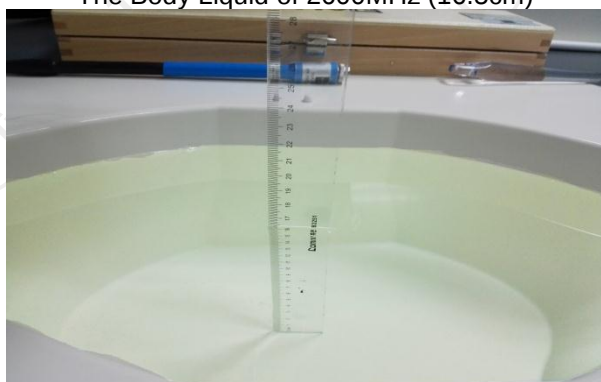
The Body Liquid of 3700MHz (15.2 cm)
