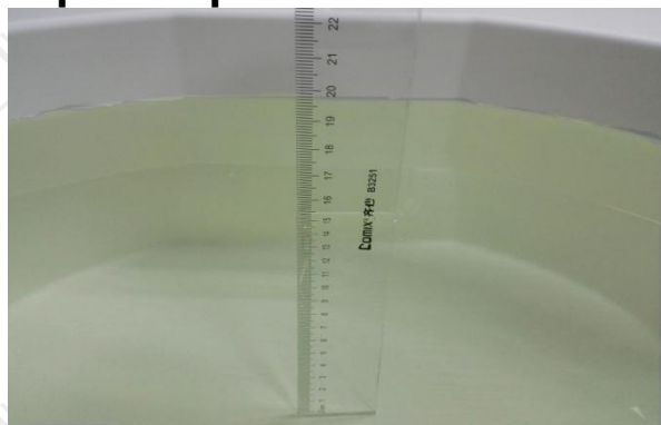
The Body Liquid of 835MHz (15.4cm)
