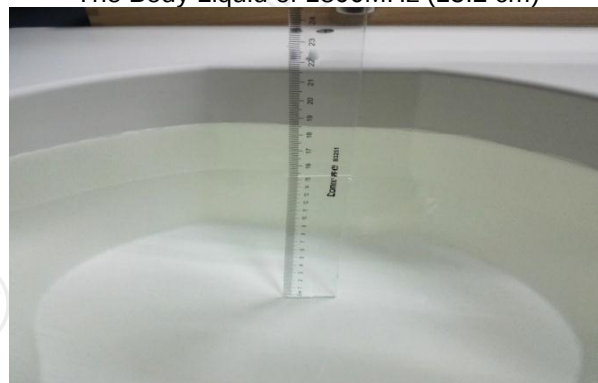
The Body Liquid of 2450MHz (15.3cm)
