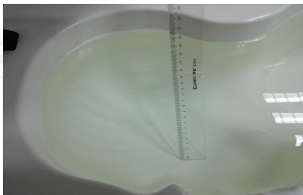
The Head Liquid of 1900MHz (15.5cm)
