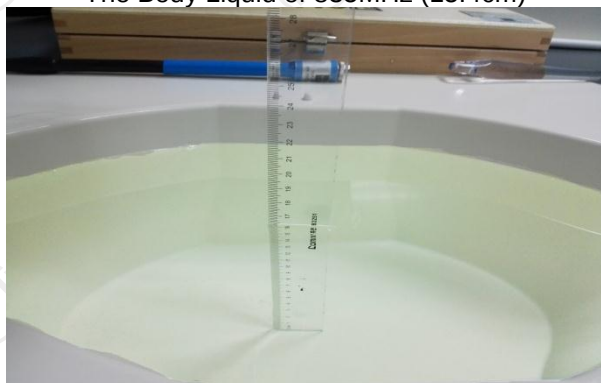
The Body Liquid of 1900MHz (16.4 cm)
