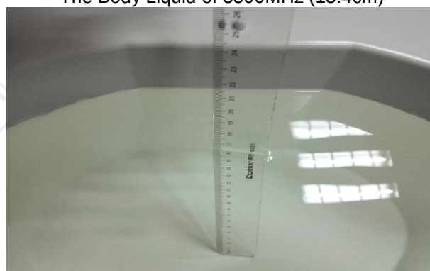
The Body Liquid of 5000-6000MHz (16.5cm)
