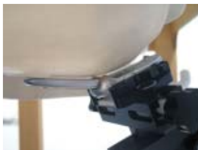
Figure 8.6 Right Head SAR Test Setup -- Cheek / Touch Position--
