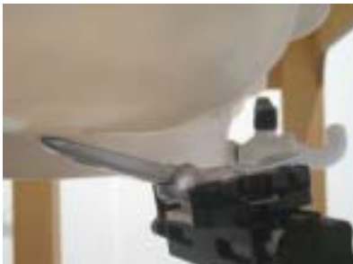
Figure 8.7 Right Head SAR Test Setup -- Ear/Tilt 15° Position--
