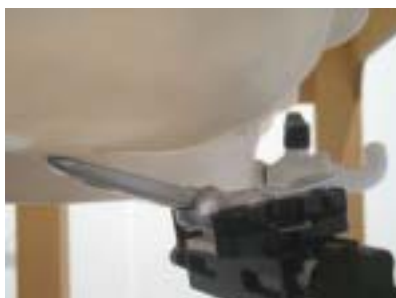
Figure 8.3 Right Head SAR Test Setup -- Ear/Tilt 15° Position--
