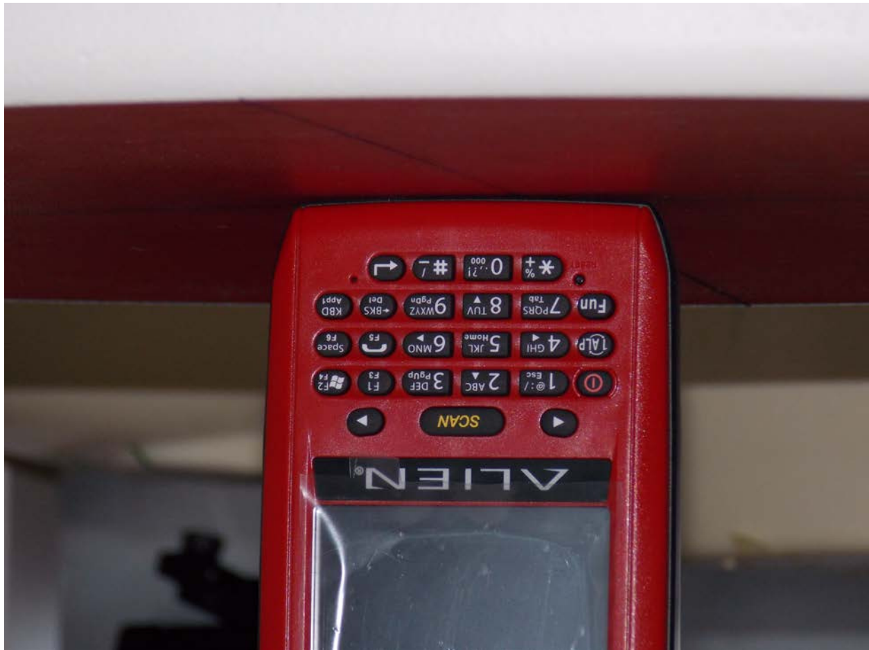
Test Position Side E Without RFID Module 0 mm Gap
