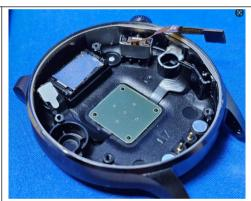
The antenna is Metal mid-frame antenna.
