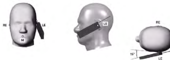
Figure 6.3 Front, Side and Top View of Ear/15° Position
