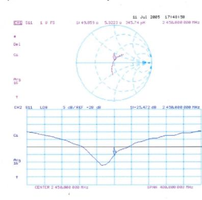
Impedance Measurement Plot for Body TSL
