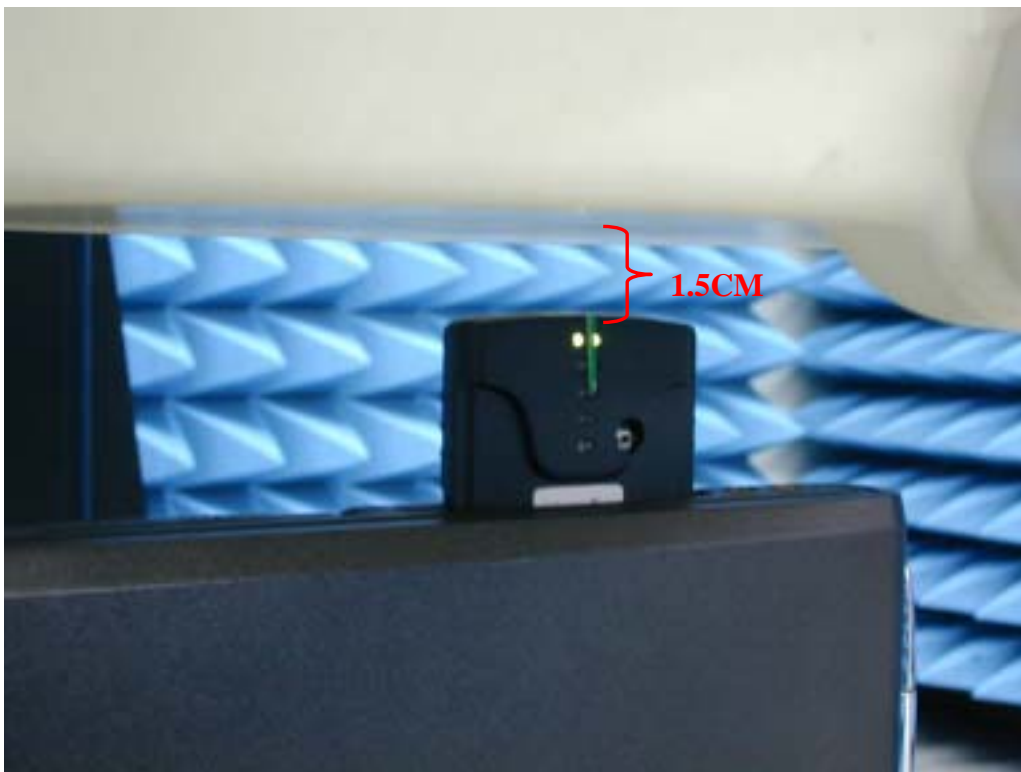
Fig.5 Photograph of the edge of the PC at 90° and at a distance of 1.5 cm from the base of the phantom
