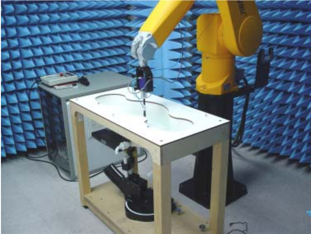
Fig.2 Photograph of the SAR measurement System
