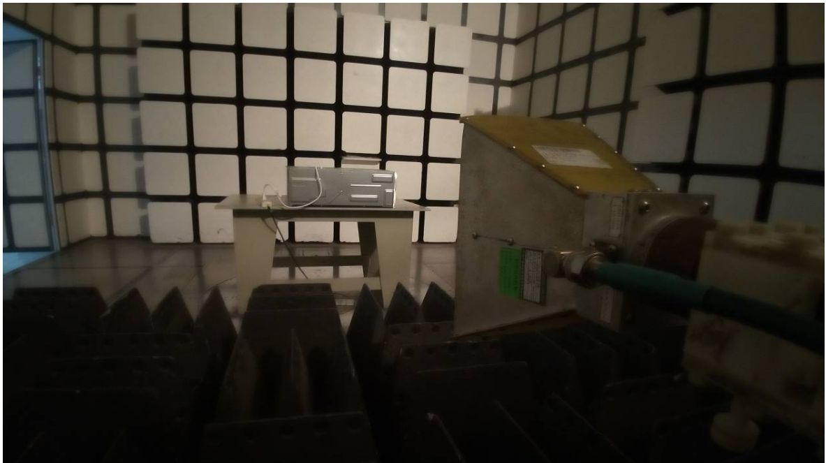
Radiated Emissions - Rear View (Above 1 GHz)
