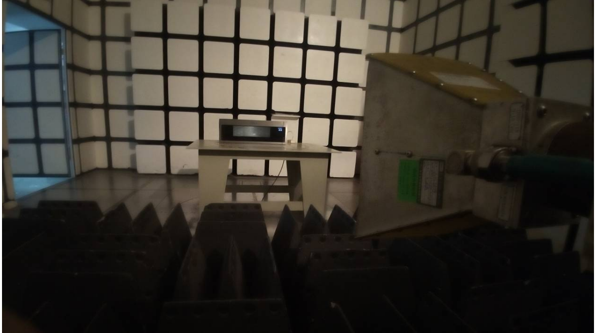
Radiated Emissions - Front View (Above 1 GHz)
