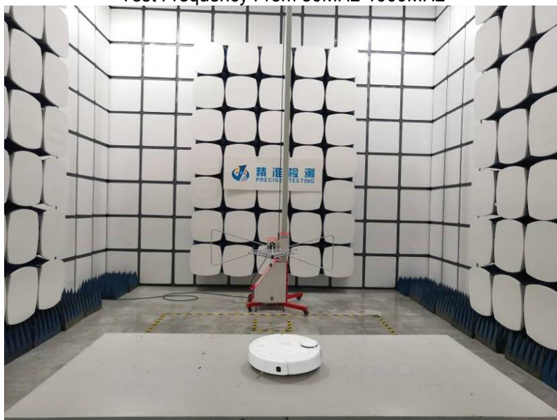
Radiated Spurious Emissions Test Frequency From 30MHz-1000MHz
