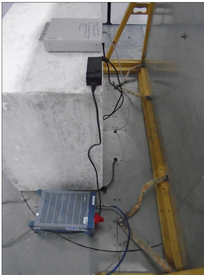
Figure 60 - AC Line Conducted Emissions
