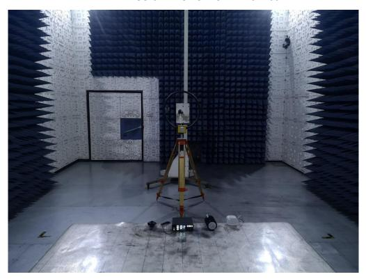
RADIATED EMISSION TEST SETUP BELOW 1GHz
