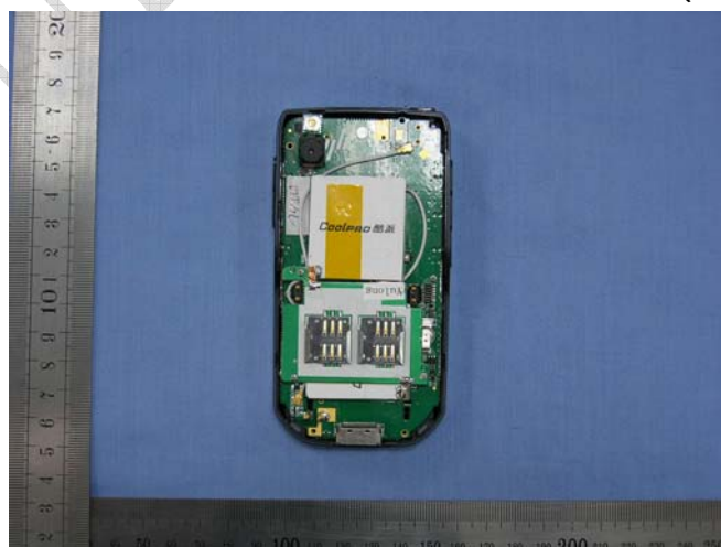
Picture 7 Back view of the internal structure, with SIM card slots
