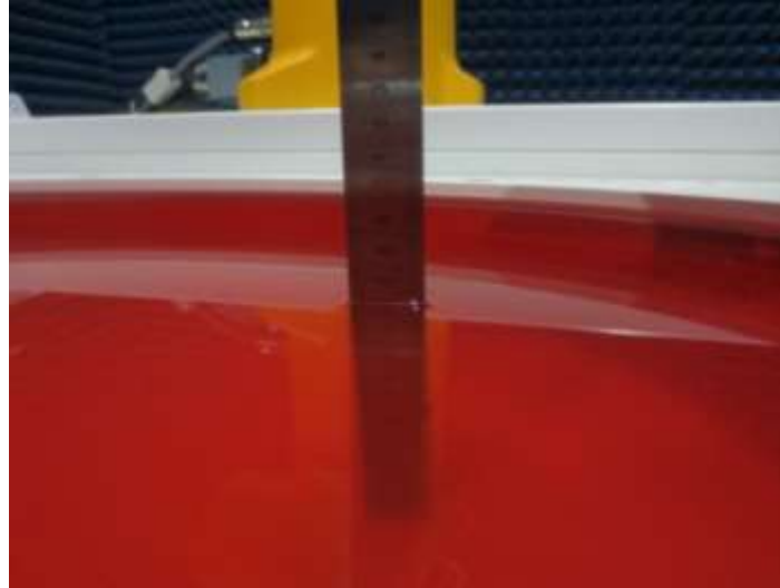
Fig. 9.6 Photo of Liquid Height for Body SAR of ELI V5.0 (2000MHz~2600MHz) (depth>15cm)
