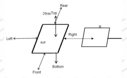
Note: Measurements should be made at 20 cm surrounding the EUT and 20cm above the top surface of the EUT.
