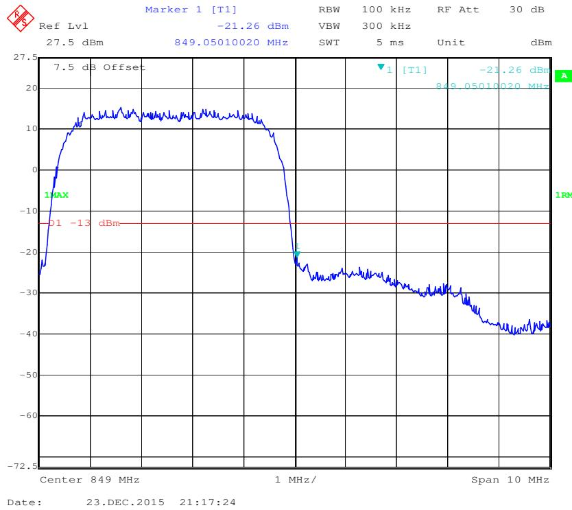
**Cellular Band, Left Band Edge for HSDPA (16QAM) Mode**
