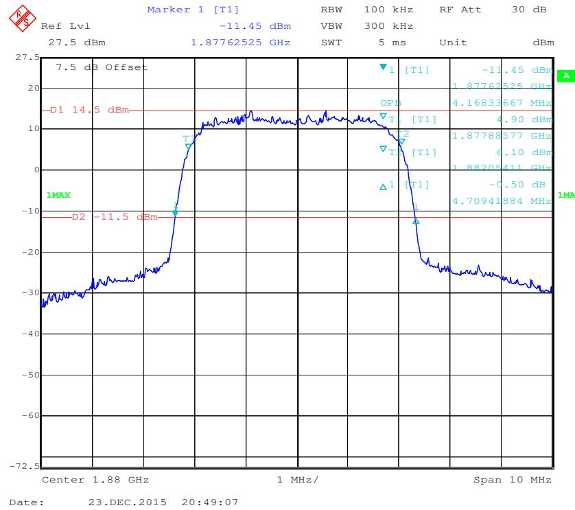
**Part 27****99% Occupied &26 dB Emissions Bandwidth for WCDMA (BPSK) Mode**
