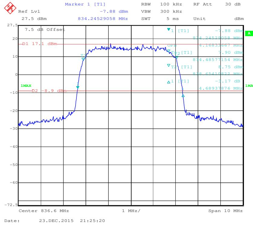
**PCS Band (Part 24E)****99% Occupied &26 dB Emissions Bandwidth for GSM (GMSK) Mode**
