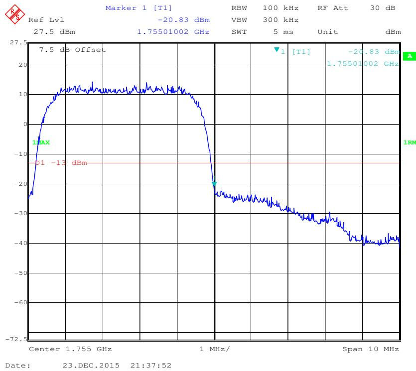
**Band IV, Left Band Edge for HSDPA (16QAM) Mode**
