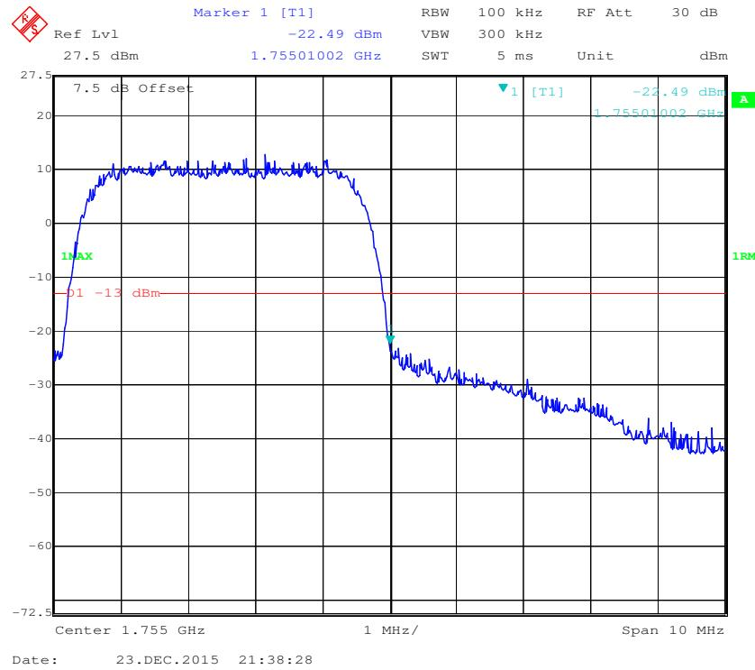
**Band IV, Left Band Edge for HSUPA (BPSK) Mode**
