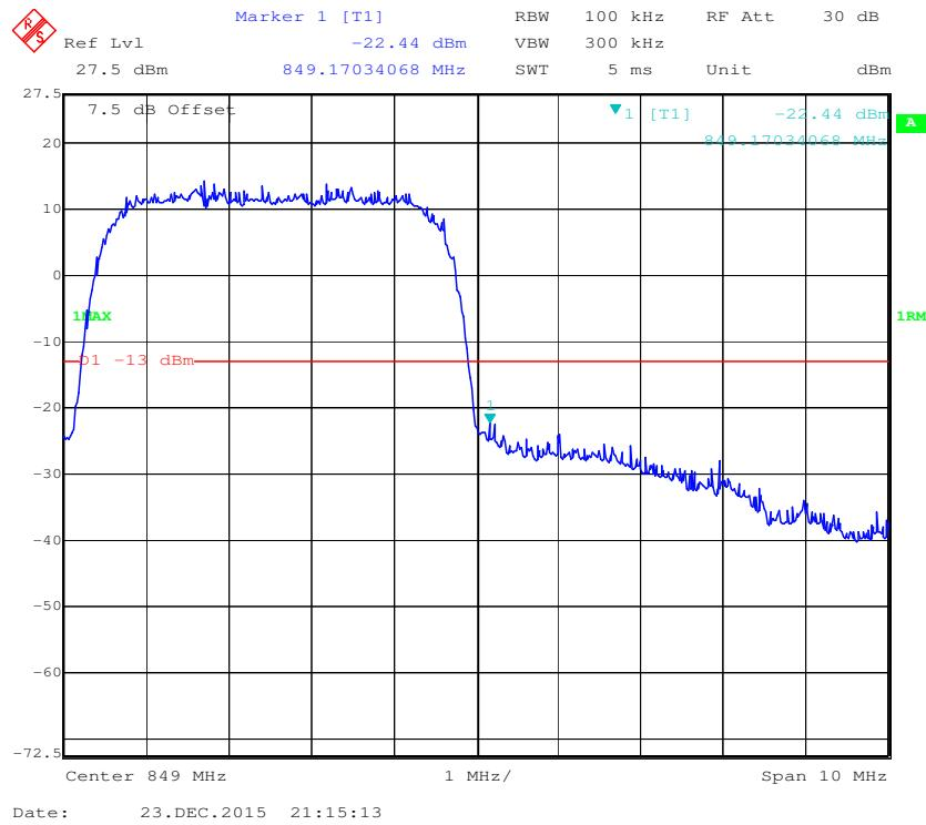
**Cellular Band, Left Band Edge for HSUPA (BPSK) Mode**
