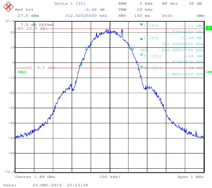
**99% Occupied &26 dB Emissions Bandwidth for EGPRS Mode**
