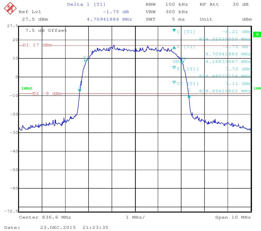
**99% Occupied &26 dB Emissions Bandwidth for HSDPA (16QAM) Mode**
