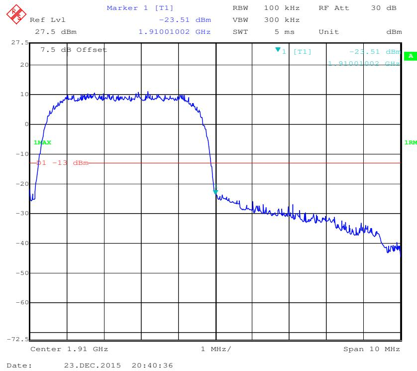
**PCS Band, Left Band Edge for HSUPA (BPSK) Mode**
