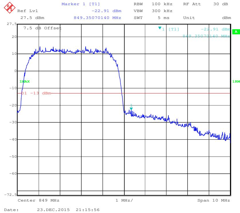
**PCS Band, Left Band Edge for GSM (GMSK) Mode**
