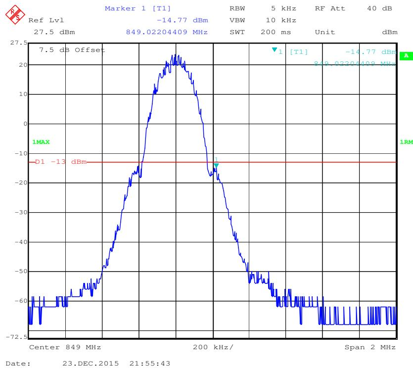
**Cellular Band, Left Band Edge for EGPRS Mode**
