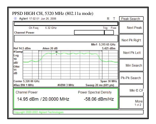
EUT: BROADCOM 802.11 ag /DRAFT 802.11n WIRELESS LAN PCI-E MINI CARD
