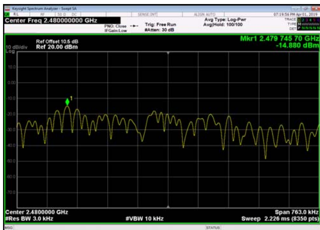
Power spectral density: 2480MHz
