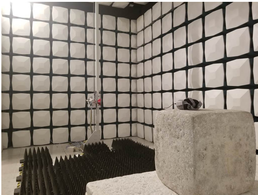
Description: Radiated Emission Test Setup for 1~18GHz
