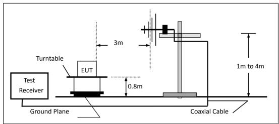
(c) For radiated emissions above 1000MHz
