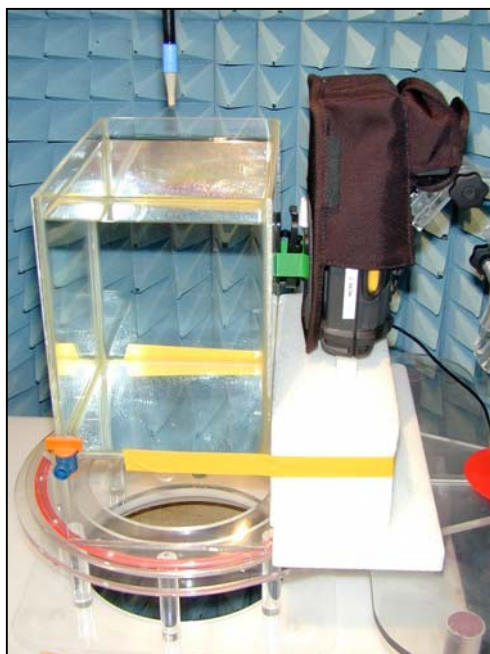
Figure 39. Positional photograph of the MC9062 With the device in a Mobile Computer Holster With the LCD side facing the rear of the Holster and the belt Clip in contact with the flat phantom.
