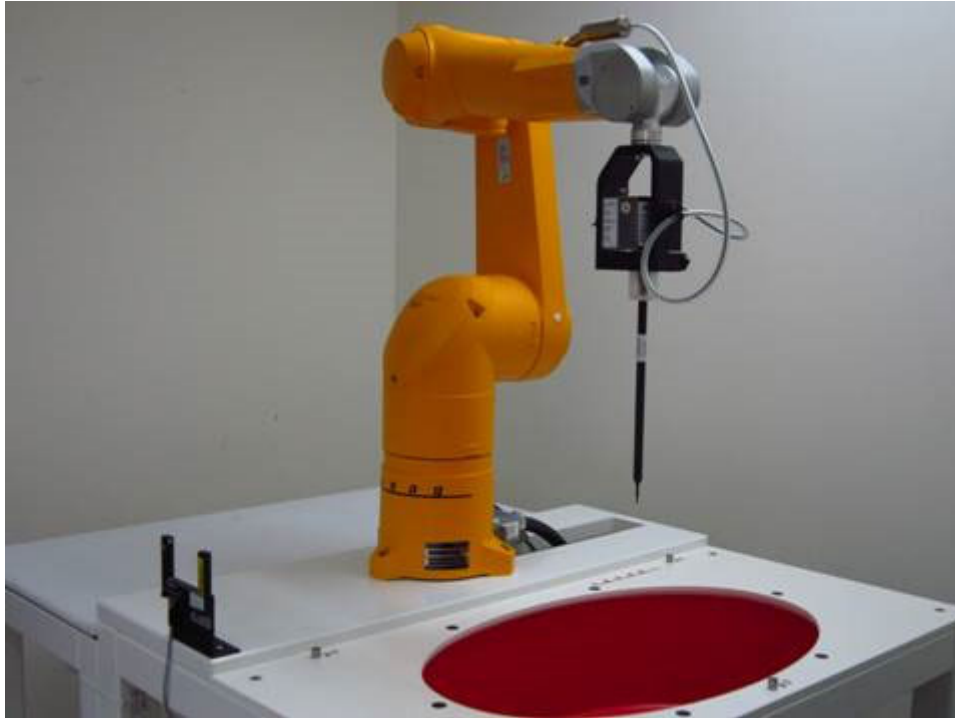
Fig.1 Photograph of the SAR measurement system
