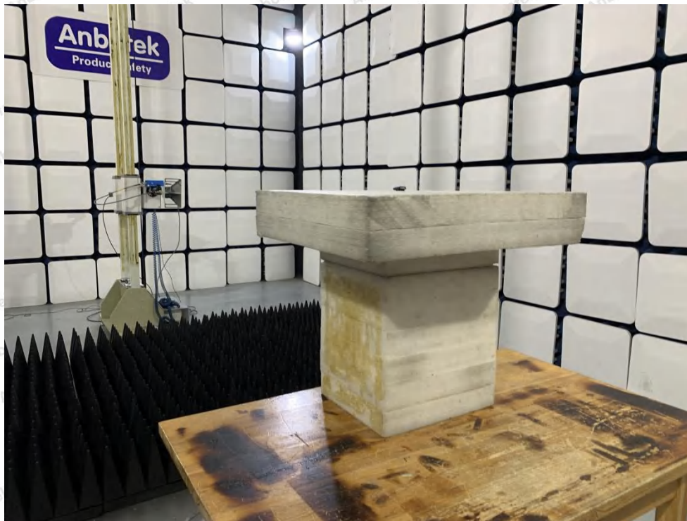
Photo of Radiation Emission Test (above 1GHz)
