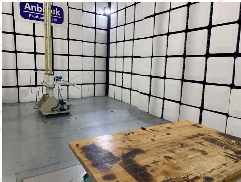
Photo of Radiation Emission Test (below 1GHz)
