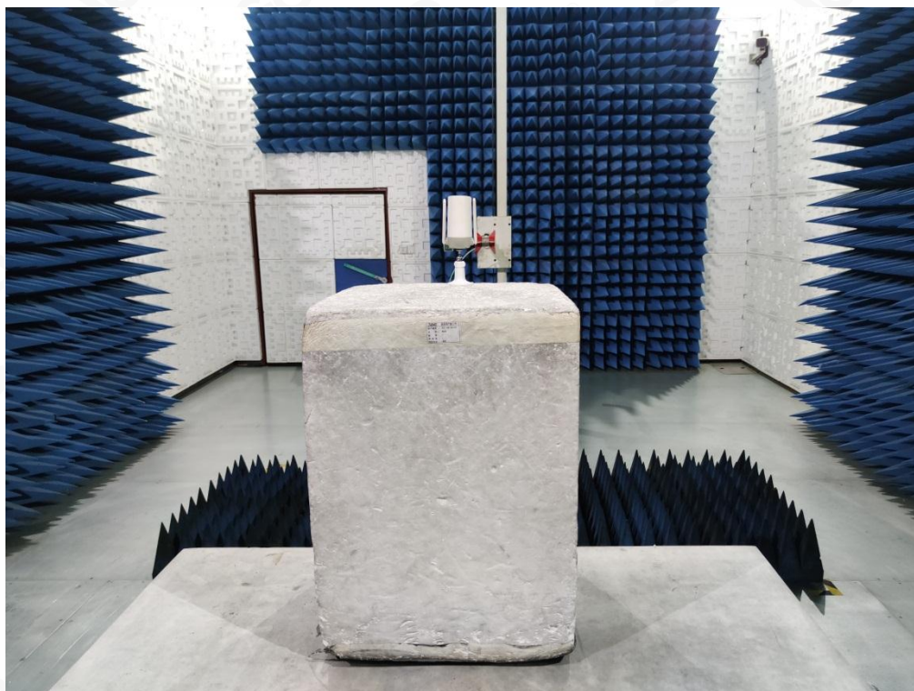
FCC RADIATED EMISSION TEST SETUP ABOVE 1GHZ
