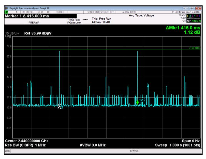
Time Between Pulses = 103 ms – Data Mode Total Duty Cycle = (580 us) / 100 ms = 0.580% The maximum peak to average ratio of -20 dB can be utilized.
