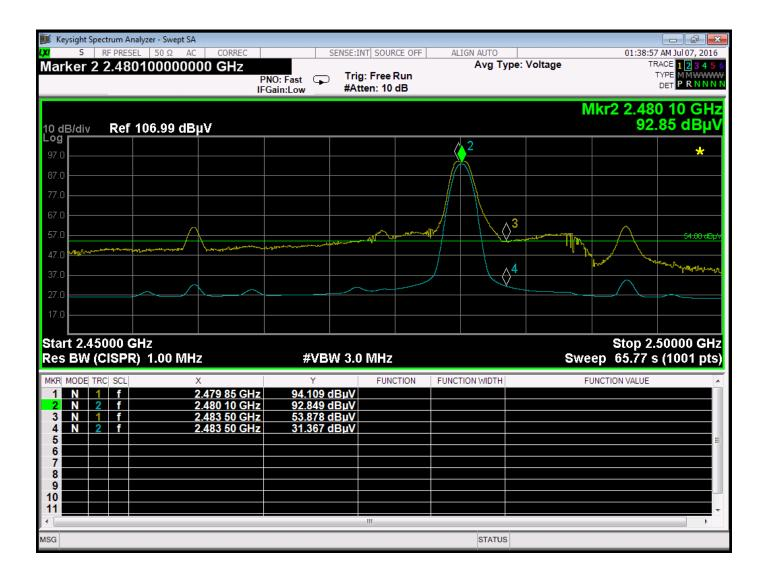
Band Edge - Horizontal Polarization - High Channel - Model: GYM3300 - X-Axis Worst Case
