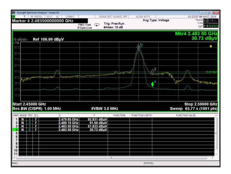
Band Edge - Vertical Polarization - High Channel - Model: GYM3300 - Z-Axis Worst Case
