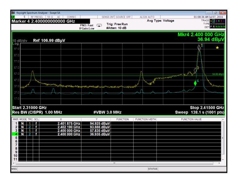
Band Edge - Vertical Polarization - Low Channel - Model: GYM3300 - Z-Axis Worst Case
