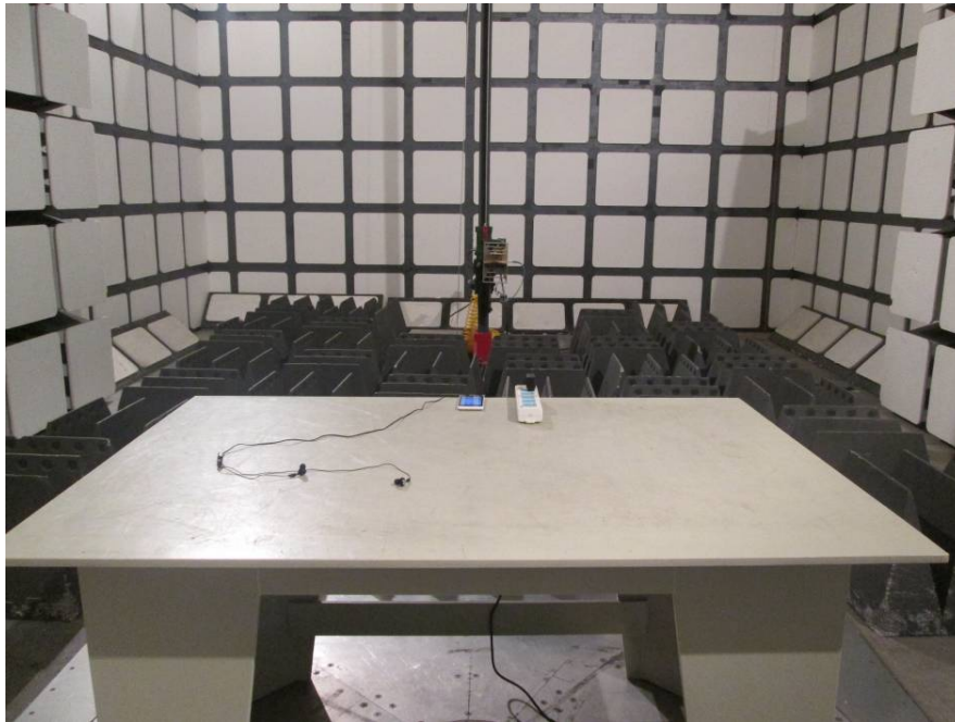
Radiated Emissions – Front View (Above 1GHz)
