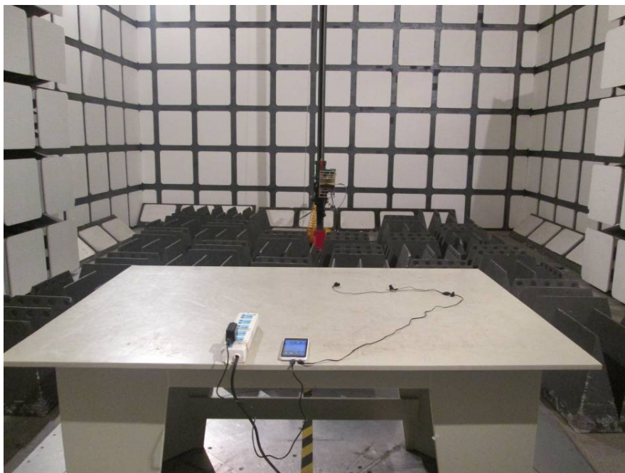
Radiated Emissions – Rear View (Above 1GHz)
