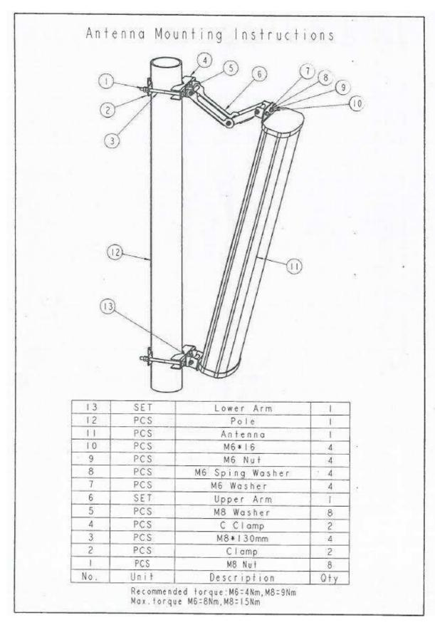
Mechanical Downtilt:  $0^{\circ} - 30^{\circ}$ Pole Diameter: 30 mm - 80 mm
