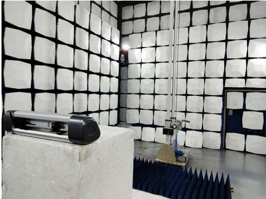
Spurious Radiated emission test view
