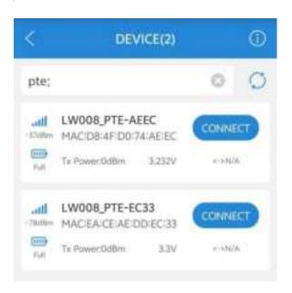
After the device is turned on, the device Bluetooth will start broadcasting. Open the MKLoRa APP and choose LW008, then you can search the LW008-PTE device by click the refresh icon. The default broadcast name of the device: LW008-PTE -XXXX.
