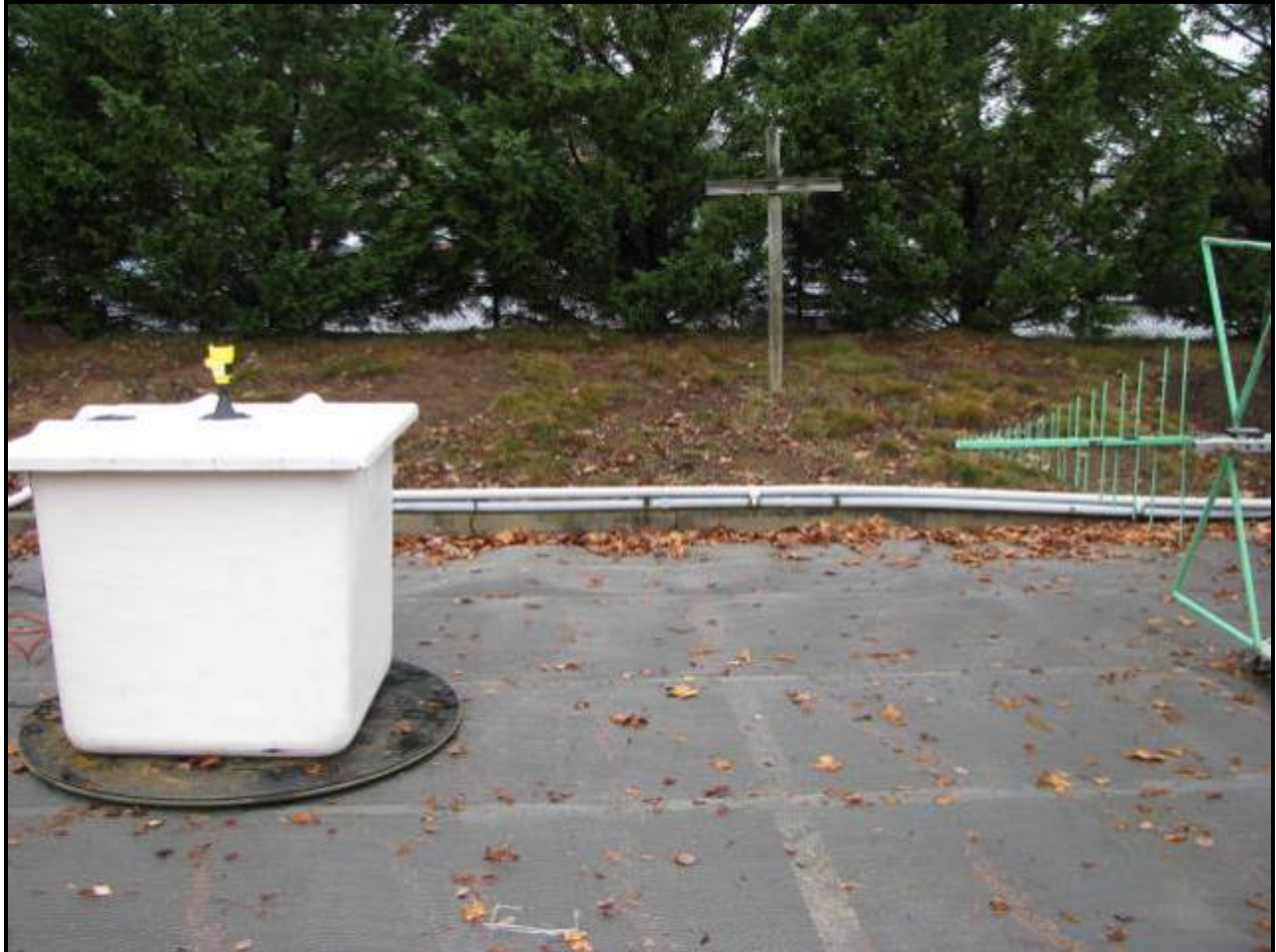
Photograph 13: Radiated Emissions – TC #1; Fiberglass Container
