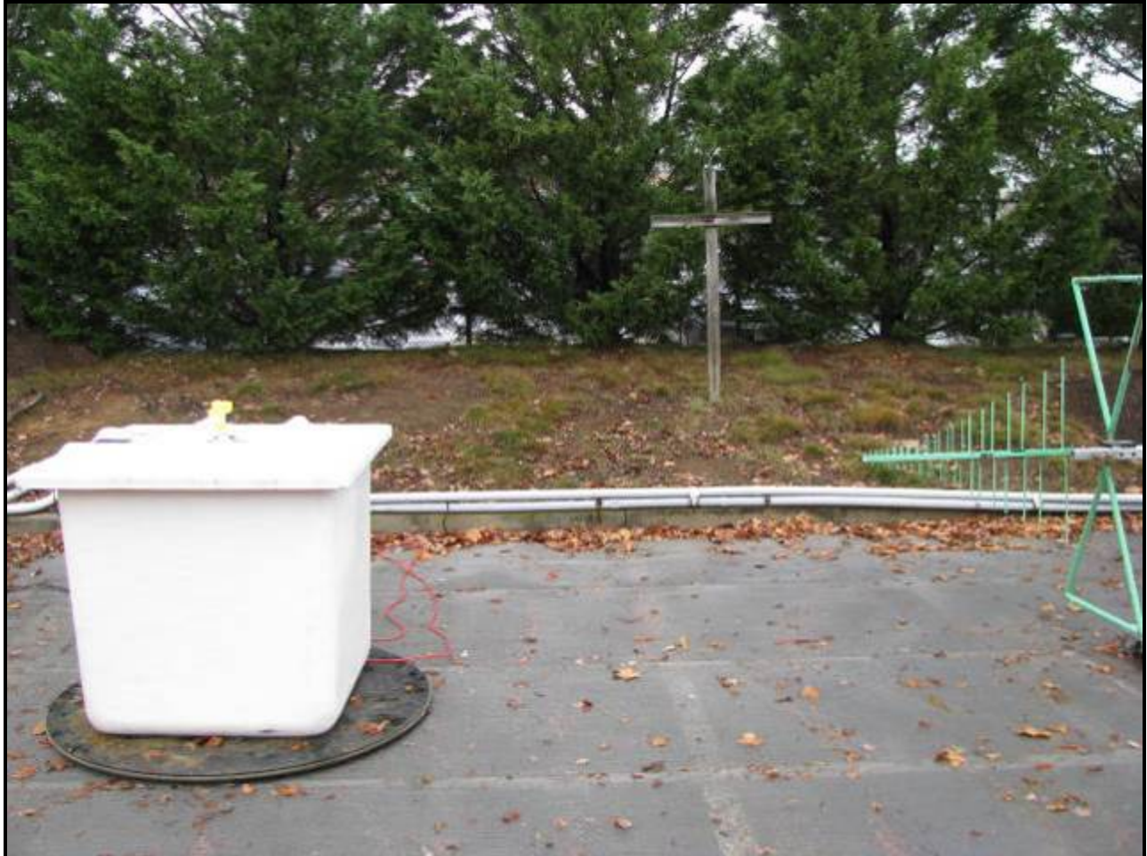
Photograph 16: Radiated Emissions – TC #2; Fiberglass Container
