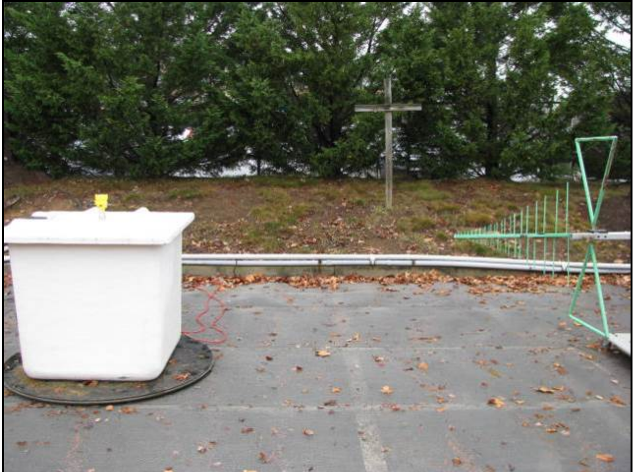
Photograph 19: Radiated Emissions – TC #3; Fiberglass Container
