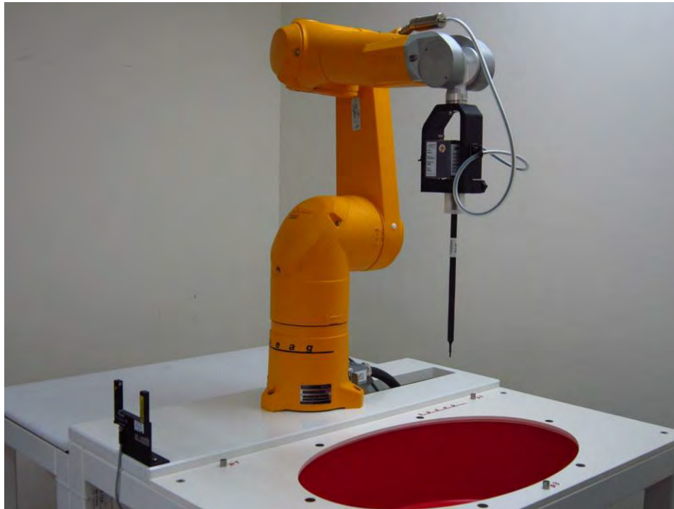
Fig.1 Photograph of the SAR measurement system
