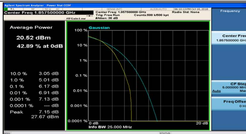
(Channel Bandwidth:15 MHz)_LCH_16QAM_75RB#0
