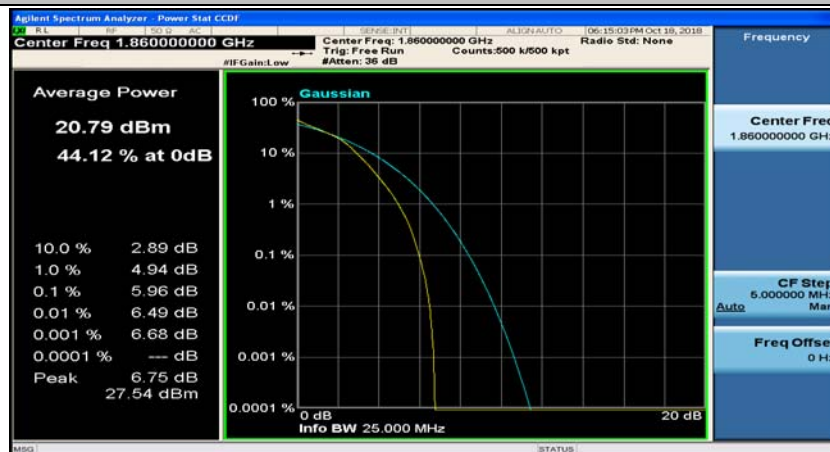
(Channel Bandwidth:20 MHz)_LCH_16QAM_100RB#0
