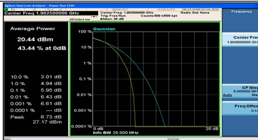
(Channel Bandwidth:15 MHz)_HCH_16QAM_37RB#18
