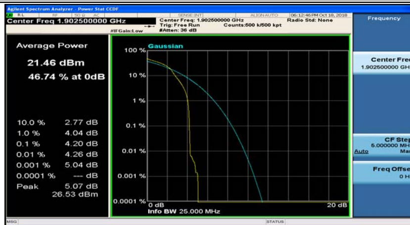
(Channel Bandwidth:15 MHz)_HCH_16QAM_37RB#0
