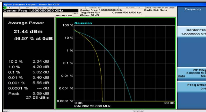
(Channel Bandwidth:20 MHz)_HCH_QPSK_50RB#25
