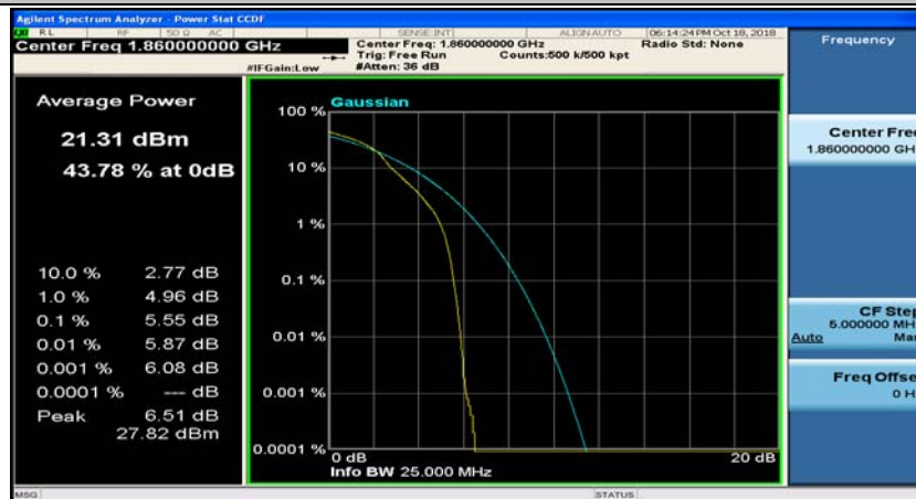
(Channel Bandwidth:20 MHz)_LCH_16QAM_50RB#0
