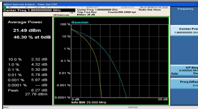
(Channel Bandwidth:20 MHz)_LCH_QPSK_50RB#50
