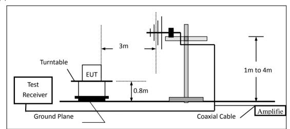
(c) For radiated emissions above 1000MHz
