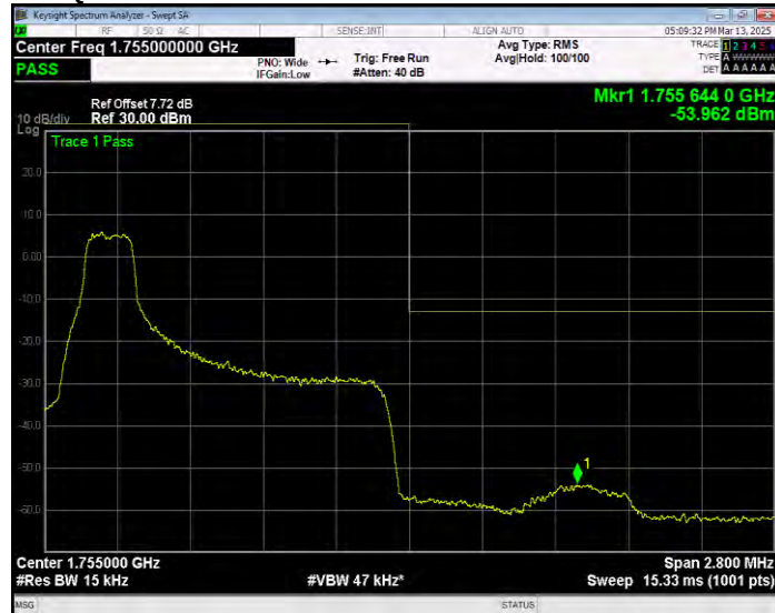
Band4 QPSK BW=1.4MHz Channel=20393 RB Size=1 Position=#0 Normal
