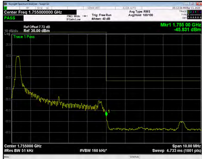
Band4 16QAM BW=5MHz Channel=20375 RB Size=1 Position=#0 Normal
