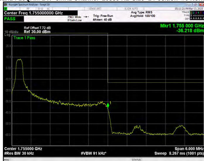
Band4 16QAM BW=3MHz Channel=20385 RB Size=1 Position=#0 Normal
