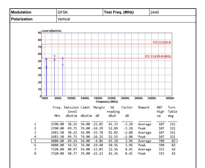
\*Factor includes antenna factor, cable loss and amplifier gain
