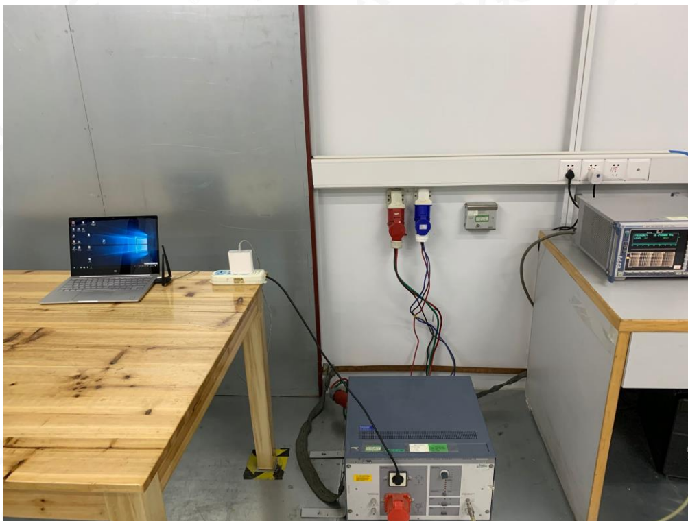
FCC RADIATED EMISSION TEST SETUP BELOW 1GHZ
