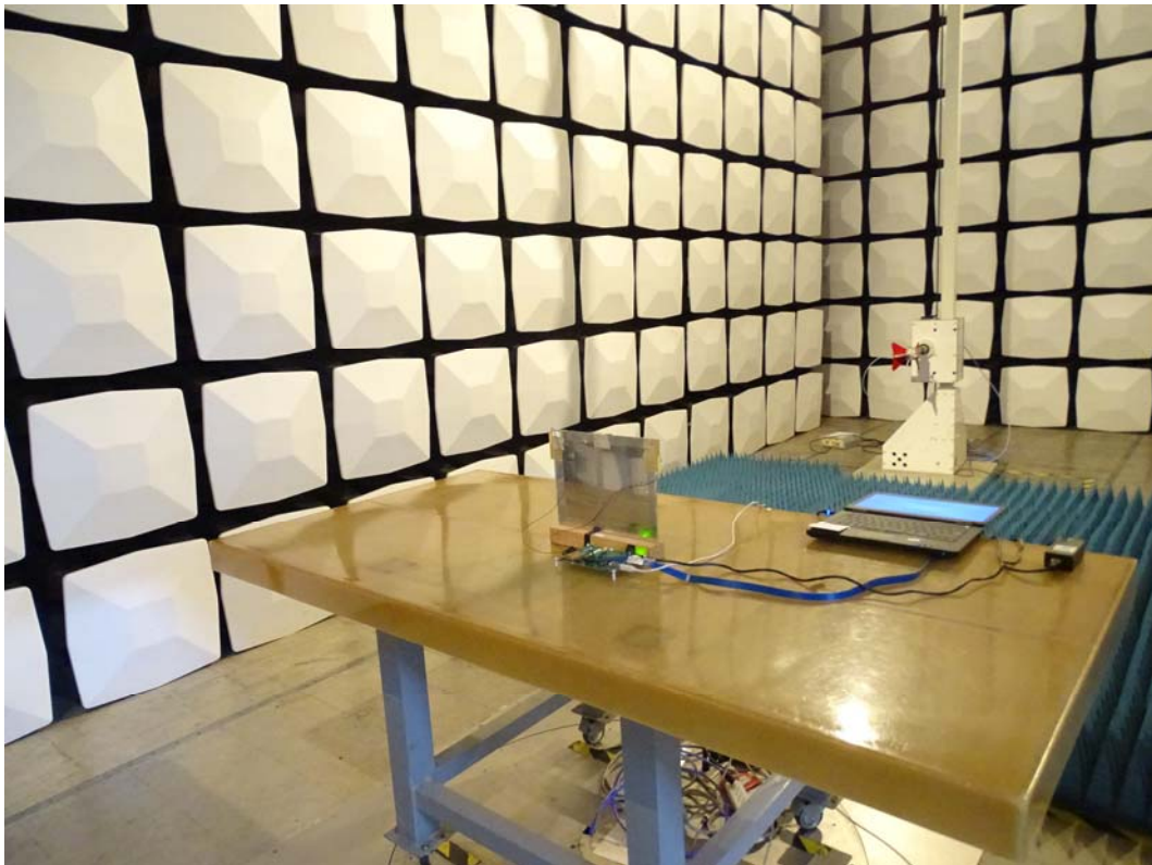
Front View of Radiated Test (Horn)
