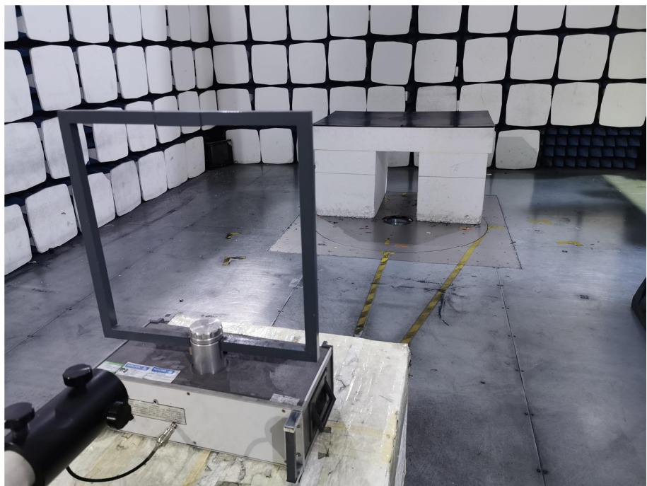
Radiation Emission Test Setup (Below 30MHz)
