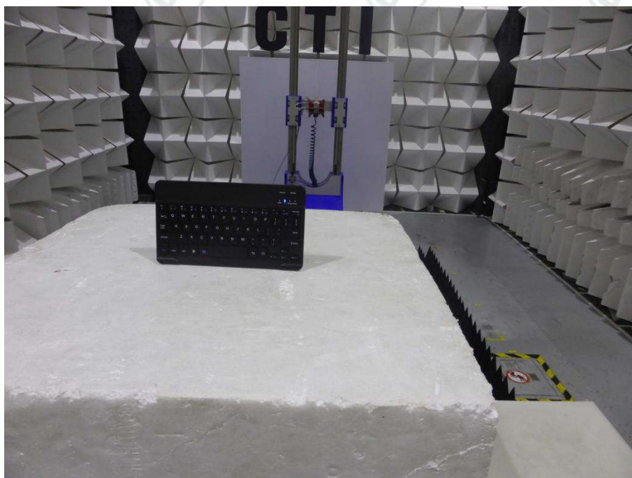
Radiated spurious emission Test Setup-2(Above 1GHz)
