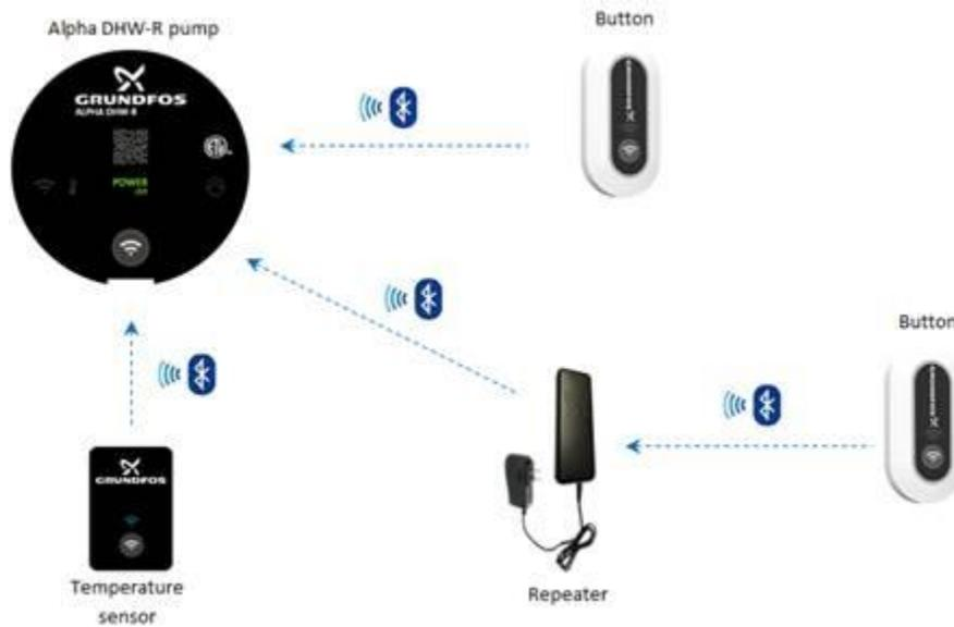
*Figure 1 – Block diagram of the HWR-D system*
