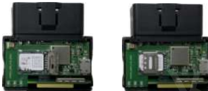
Figure 5: SIM Card Installation
