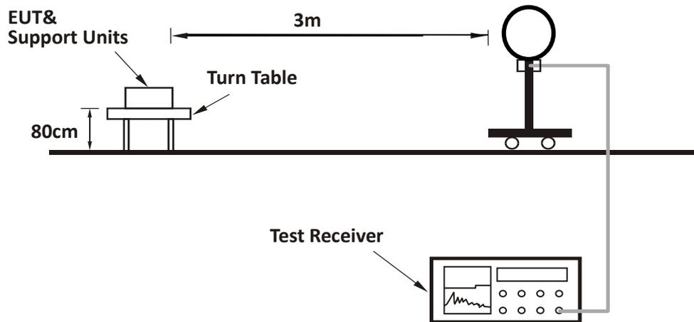
For Radiated emission 30MHz to 1GHz:
