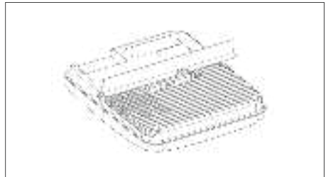
5. Ensure that all the mounting posts on the rear-side of the AP are snapped in to the respective notches on the bracket.
