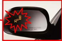
✓ Warning level 1 : Lamp turn on✓ Warning level 2 : Lamp blink and sound
