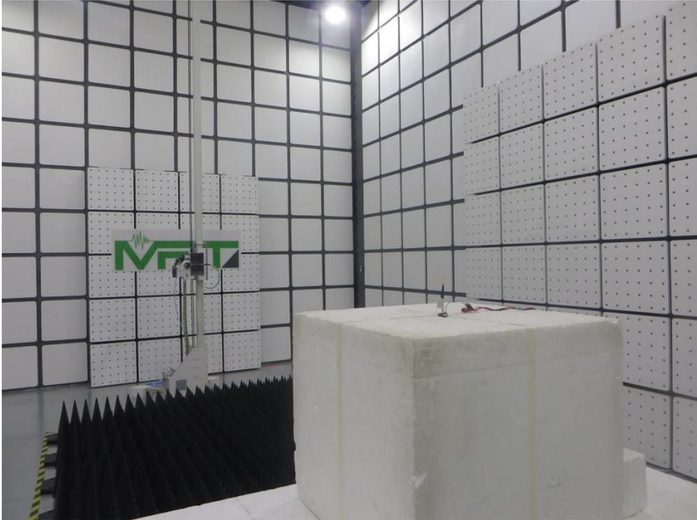
Description: Radiated Spurious Emissions Test Setup for 18GHz ~ 25GHz
