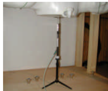
Figure 12.1 Dipole Validation Test Setup
