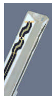
Figure 3.2 Probe Thick-Film Technique
