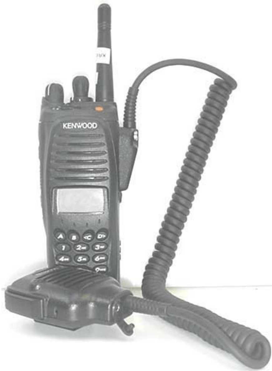
DUT with Speaker-Microphone Audio Accessory (P/N: KMC-25)
