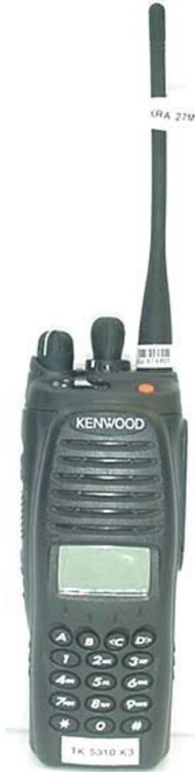
Front of DUT (KRA-27M Antenna)
