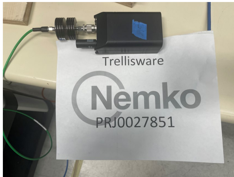
Figure 9 – Test setup, antenna conducted port.
