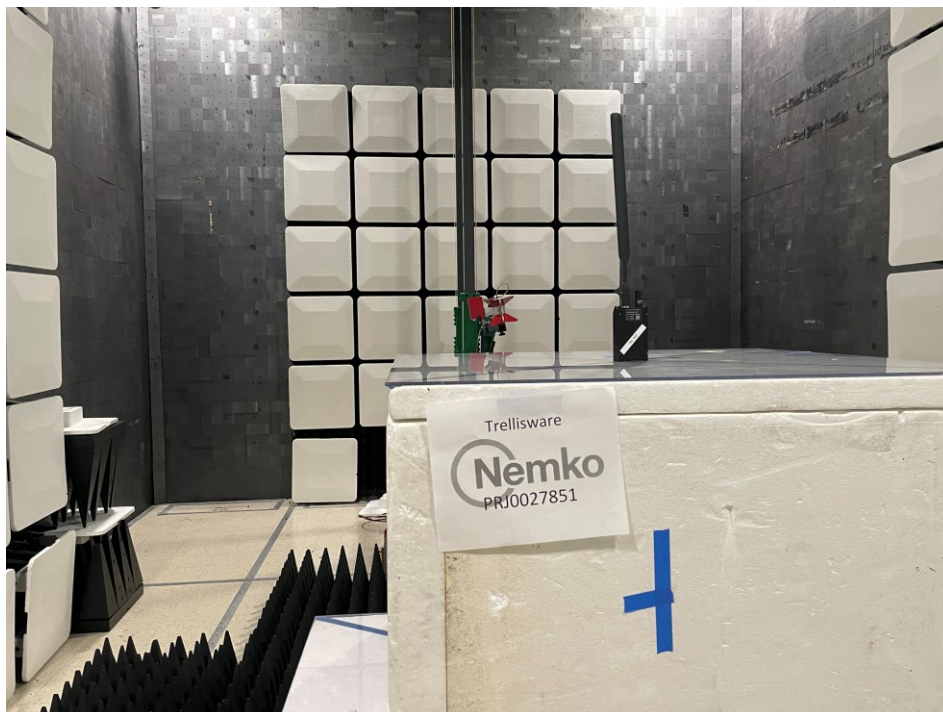
Figure 5 - Radiated emissions above 1 GHz (1 – 18 GHz), rear view.
