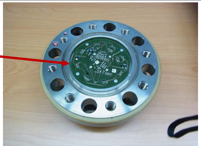
The rotor includes 4 PCB*
